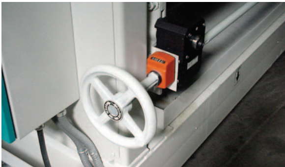
Single Handwheel Doctor Roll Adjustment
